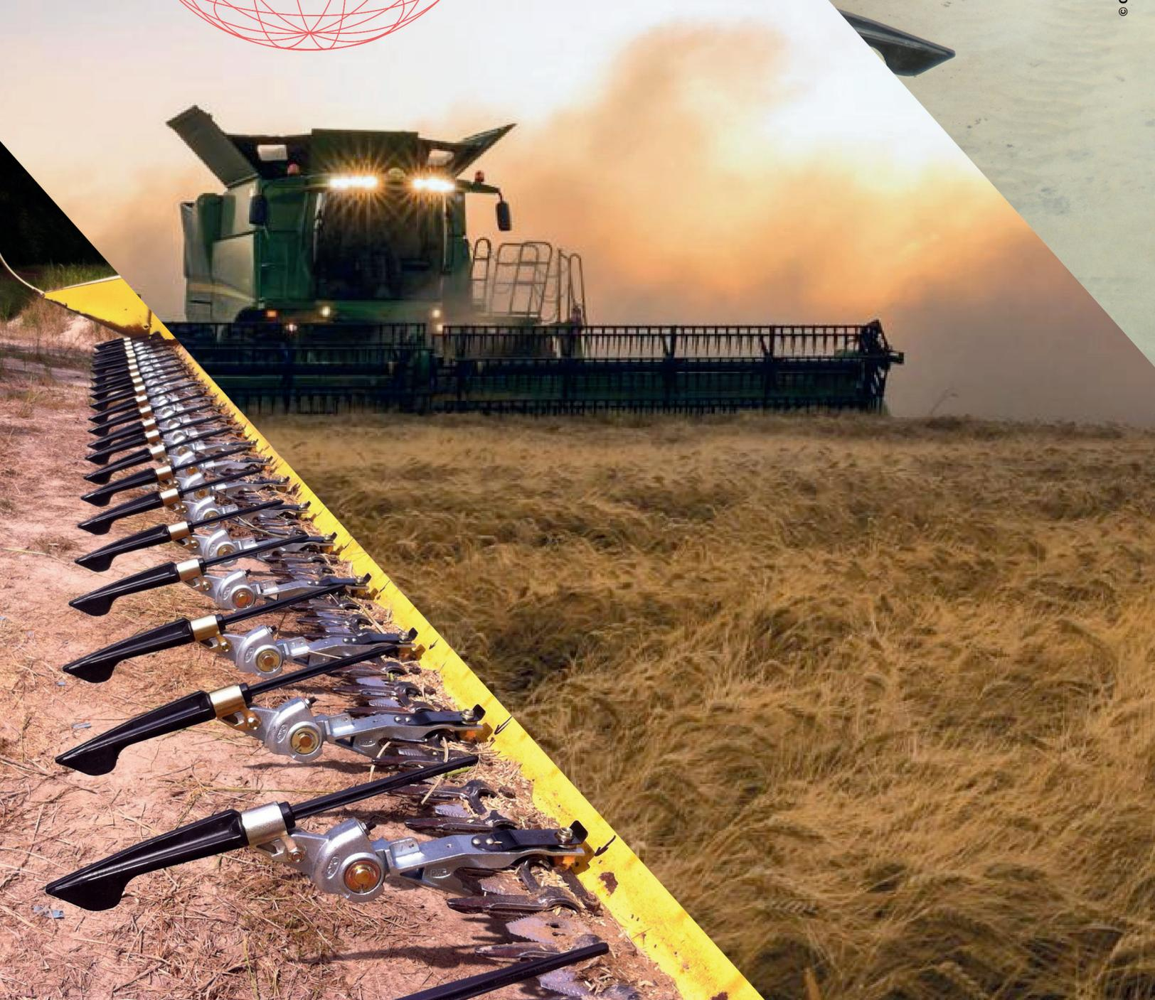
All Flexxifinger® crop lifters attach with our Flexxifinger® patented QD™ (quick detach) nut assembly which enables them after initial installation to be removed and reinstalled within minutes.
