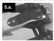
a. Slide the lifter snout over the guard with the rail spring side up. Push the lifter rail into the rail slot on the QD™ nut. The rail spring will pop into place under the safety groove. See Diagram 3 and 4. Install lifters on all remaining QD™ nuts and check each lifter to ensure there is adequate clearance from the knife.
