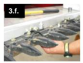
f. Install the remaining QD™ nuts on the rest of the header using the first-installed QD™ nut as a guide. When necessary to install a QD™ nut assembly on a knife hold down, the number of washers required will need to be reduced by the thickness of the knife hold down. Do not torque the QD™ nuts just yet.
