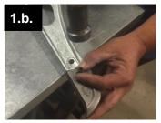
b. Insert the roll pin into the hole of the shoe. Using a hammer, pound the roll pin into the hole until the end of the roll pin is flush on either side of the shoe. If installing the 20235 2-hole long shoe, repeat this step for installing the other roll pin.
