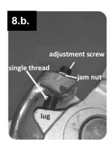
b. Turn the adjustment screw to adjust the lifter to the desired angle, keeping in mind that a half-turn of the adjustment screw affects the downward travel angle of the lifter by about 5 degrees. The recommended approximate minimum set screw adjustment is outlined in the chart below:
