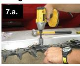
a. Remove all lifters and tighten all QD™ nuts to 60ft-lb/81Nm torque. Once installed, the QD™ nuts can remain on the header.
