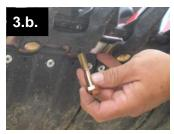
b. Insert the 10mm x 55mm bolt from the bottom of the header.
