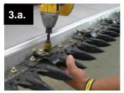
a. Starting 12"/30cm from the right side of the header and every 12"/30cm across the header, remove the guard nut and bolt from the guards. (Please note that the setup for crops seeded in rows requires specialized spacing. Please contact us for setup instructions in this case.)
