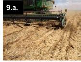
a. Whenever possible prior to installing the crop lifters on the header, combine approximately 100 feet without the lifters to adjust the header angle, reel speed/height, header height, etc. to achieve optimal settings of the header alone. Once the lifters are installed, drive slowly over the path that has been harvested and observe whether or not the lifters need to be adjusted.
