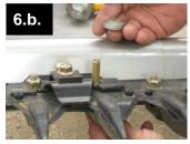
b. If any one lifter is not in line with the others, remove that lifter. Remove the QD™ nut and adjust the number of washers as required (either by adding or subtracting washers) so that the base of the accessory plate is level with the others. Repeat for each lifter that is not level with the others until the base of each accessory plate forms a straight line as shown in image 6.a. above.
