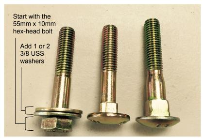
NOTE: Using the above configurations, the hex-head bolt may wear over time, in which case it will be impossible to remove without cutting or grinding it off. The hex-head will also catch plant material and rocks under the bolt.
