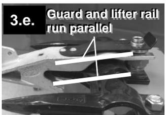
a. Starting 12"/30cm from the right side of the header and every 12"/30cm across the header, remove the guard nut and bolt from the guards. (Please note that the setup for crops seeded in rows requires specialized spacing. Please contact us for setup instructions in this case.)
