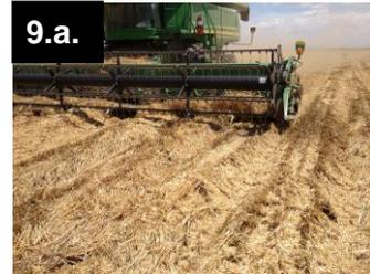
a. Whenever possible prior to installing the crop lifters on the header, combine approximately 100 feet without the lifters to adjust the header angle, reel speed/height, header height, etc. to achieve optimal settings of the header alone. Once the lifters are installed, drive slowly over the path that has been harvested and observe whether or not the lifters need to be adjusted.
