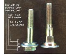
FOR ANY OTHER HEADER REQUIRING A CARRIAGE BOLT (32312 & 32314):
