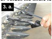
a. Slide the lifter snout over the guard with the rail spring side up. Push the lifter rail into the rail slot on the QD™ nut. The rail spring will pop into place under the safety groove. See Diagram 3 and 4.
