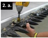
a. Starting 12"/30cm from the right side of the header and every 12"/30cm across the header, remove the guard nut and bolt from the guards. (Please note that the setup for crops seeded in rows requires specialized spacing. Please contact us for setup instructions in this case.)
