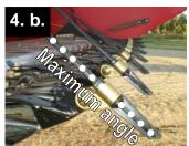
o. The finger should be set to a maximum 25 degrees from the ground and set so in the event that the finger touches the ground, the back half of the tip will make contact, as shown in Diagram 5. Generally speaking, less of an angle is usually better for lifting the plant. Ideally, the lifters should be set so that the tip of the nylon finger is about ½"/13mm to ¾"/19mm above the ground.
