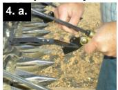
a. Loosen the receptor's lock nut from the carriage bolt and adjust the angle of the nylon finger.
