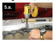
a. Tighten all QD™ nuts to 60ft-lb (81Nm) torque. Once installed, the QD™ nuts can remain on the header, even when the crop lifters are not being used.
