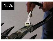
a. Using a 3/4" (19mm) wrench, loosen the adjustment bolt.
