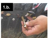
b. Insert the provided M10 hex head bolt from the bottom of the header, or the correct Flexxifinger® carriage bolt, if purchased. If a carriage bolt is needed but not on hand, use the configuration pictured above to mimic a carriage bolt.
