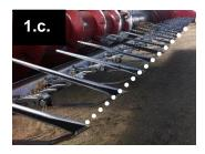
c. Set all the lifters to be the same angle; they should form a straight line when you look down the row. It is important that all lifters are working in unison. Tighten the adjustment bolt on all lifters.
