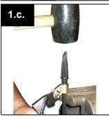
c.Use a rubber mallet or a hammer to tap the nylon finger until it has fully seated into the receptor. Notice: The fit is very snug. It helps to spray the finger with multipurpose lubricant. If it is difficult to push the finger into the receptor, check that the flat sections of the finger and receptor are not misaligned. Attempting to force the finger into the receptor may cause damage to the finger.
