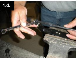
d.Once the finger is fully seated, rotate it 90 degrees with pliers or a wrench to lock it into place. If it is hard to turn, it may not be fully seated.
