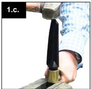
c.Use a rubber mallet or a hammer to firmly tap the nylon finger, until it has bottomed completely into the receptor.
