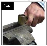
a. Holding the lifter in your hand, rest the back of the receptor between and ON TOP of the jaws of a vise, so the receptor spans the distance between the jaws.
