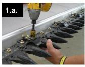
a. Starting 6"(15cm) from the right side of the header and every 12"(30cm) across the header, remove the guard nut and bolt from the guards.
