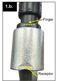
b. Slide the nylon finger tail down into the front of the receptor. Match up the flat section of the receptor with the flat section on the finger body, like a key into a lock.
