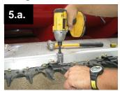
a. Tighten all QD™ nuts to 60ft-lb (81Nm) torque. Once installed, the QD™ nuts can remain on the header, even when the crop lifters are not being used.
