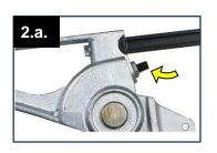
a.Loosen the jam nut. Turn the adjustment screw to adjust the lifting angle. Set the lifter to a maximum of 22 degrees from the ground.
