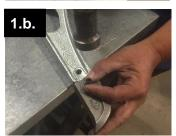
b. Insert the roll pin into the hole of the shoe. Using a hammer, pound the roll pin into the hole until the end of the roll pin is flush on both sides of the shoe. When installing the long shoe, repeat this step for installing the second roll pin.
