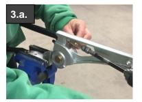
a. Tighten the rail of the crop lifter in a vise. Insert the round tenon of the nylon tail into the round hole at the back of the arm, with the rounded step of the tail fitting into the groove. Insert the self-tapping screw into the hole on the other side of the arm. Use a driver outfitted with an extension and a  $\frac{5}{16}$  (8mm) socket to drive the screw into the tail.
