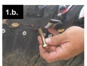
b. Insert the provided M10 hex head bolt from the bottom of the header, or the correct Flexxifinger® carriage bolt, if purchased. If a carriage bolt is needed but not on hand, use the configuration pictured above to mimic a carriage bolt.
