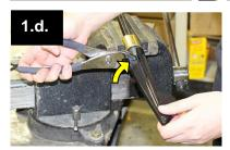
d. Once the finger is fully seated, rotate it 90 degrees with pliers or a wrench to lock it into place. If it is hard to turn, it may not be fully seated.
