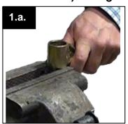
a. Rest the back of the receptor between and ON TOP of the jaws of a vise, so the receptor spans the distance between the jaws. You may remove the receptor from the lifter if necessary.
